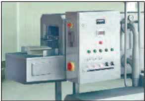
5/ Mould washing Lavado de moldes
