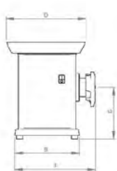
P-22. Production \pm 300 kg/h. Motor Power 1.5HP. P-32. Production \pm 425 kg/h. Motor Power 2.5HP.
