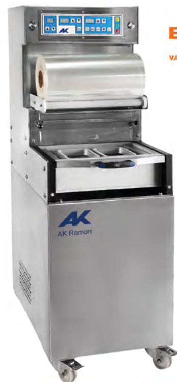
TS-550 maximun sealing surface: 320x260 mm Power: 1.500 W Requires compressed air.
