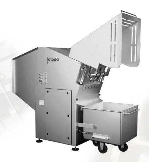
TBG480 machine for cutting frozen blocks of meat or other products at -20° C. The clean cut and size of the pieces obtained from the block make them suitable for subsequent processing in the mincer and bowl cutters, thereby reducing the time and effort required by these machines.
