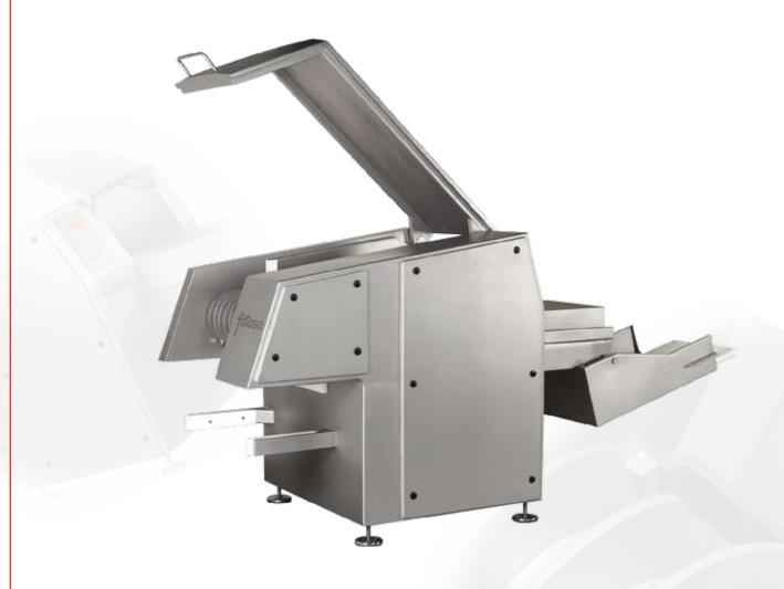
Flaker of frozen blocks CBC HP is a machine designed to cut frozen blocks of meat or other products at -20°C, by means of a rotating 4-blade roller, this produces pieces of irregular shapes and sizes depending on the type and temperature of the product.
